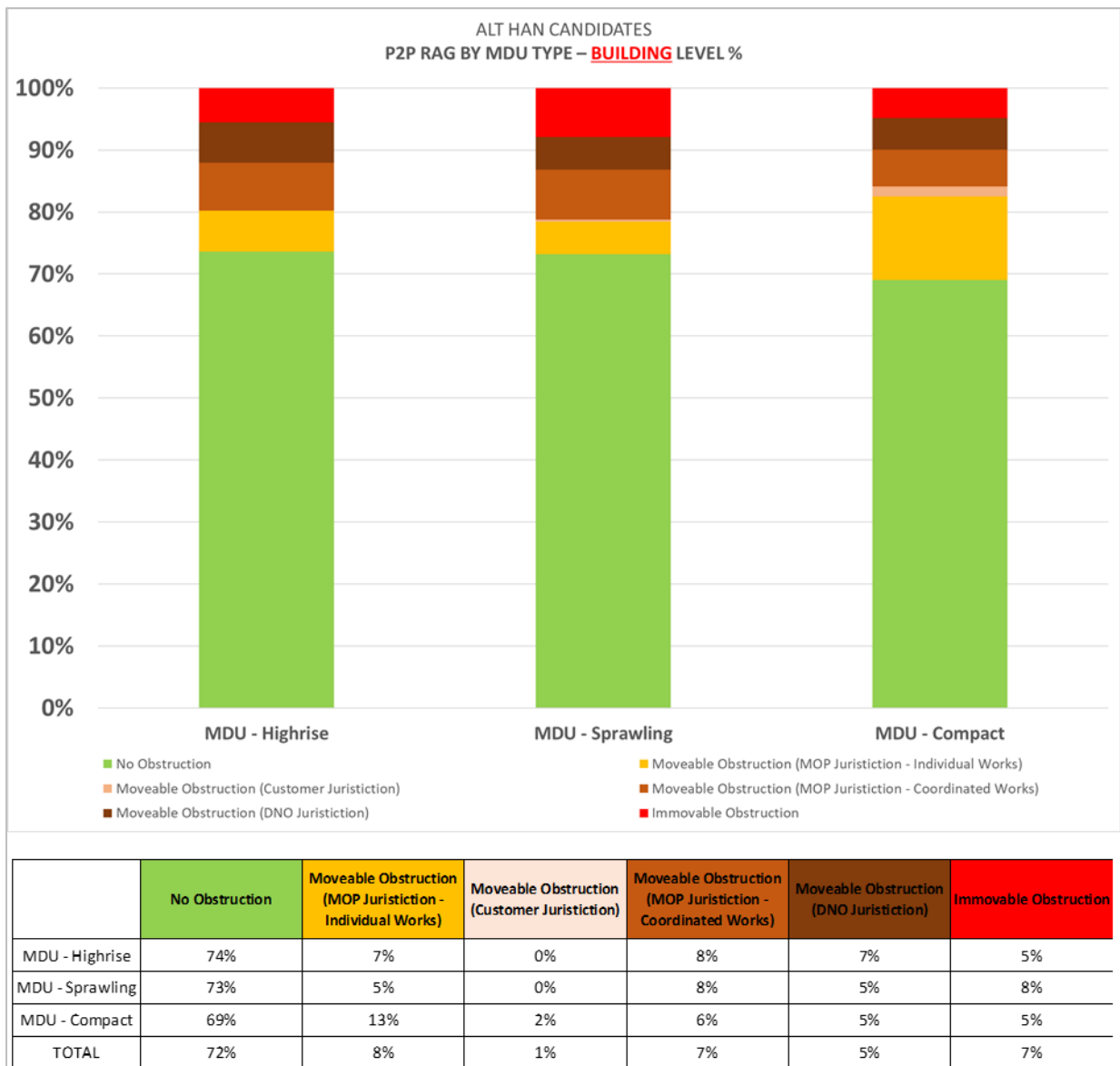
Figure 1 Results of the Alt HAN Co CMR photographic analysis of 2500 sample MDUs, split by MDU Highrise, MDU Sprawling and MDU Compact
